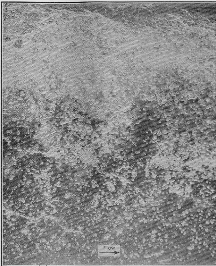
FIG. 3.—PROFILE OF PARTLY AERATED FLOW (EXPOSURE: 1/50,000 SEC)
