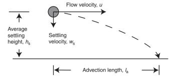
**Figure 3 | Definition sketch of the advection length scale.** The advection length scale is defined as the average horizontal distance travelled by a sediment particle before it settles to the bed (Methods, Fig. 2).
