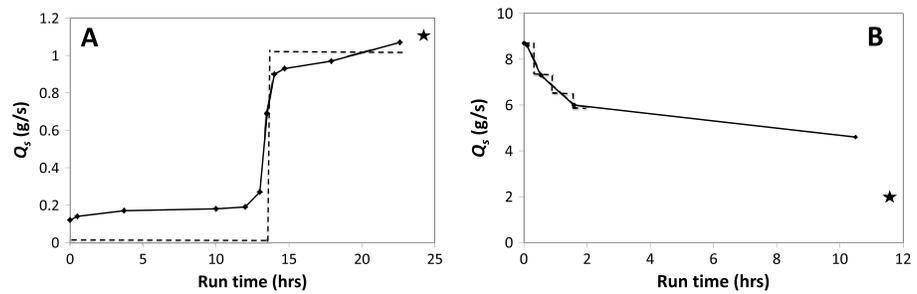
**Figure 6.** Numerical model output of sediment flux ( $Q_s$ ) at  $x = -4.5$  m as a function of time for A) Experiment 3 (low-flow transient run) and B) Experiment 4 (high-flow transient run). The dashed lines show the discretization of sediment feed rate that was used in the flume experiments. Experiment 4 was only run until  $t = 1.72$  h. The stars indicate the sediment supply from the equilibrium experiments.
