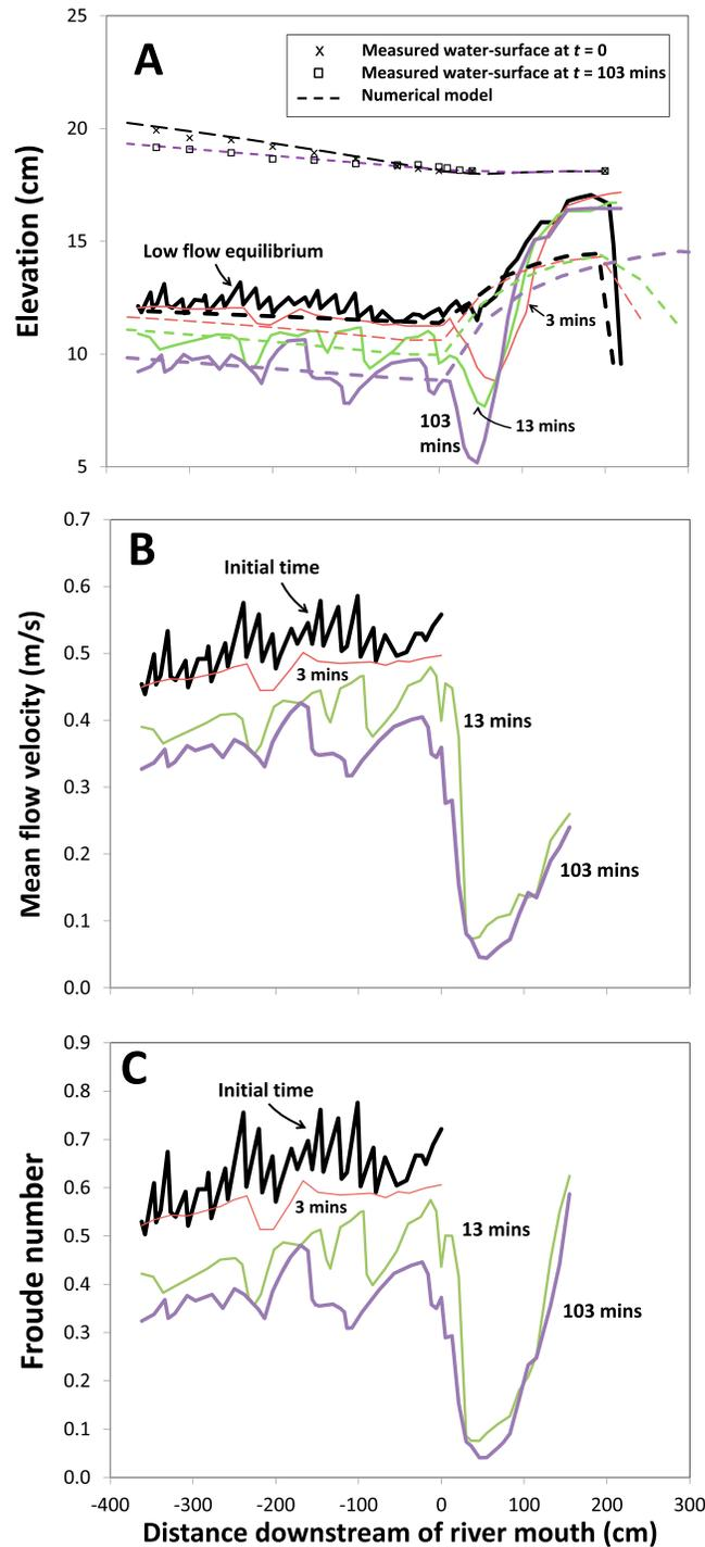
**Figure 8.** Experimental results from Experiment 4 (high-flow transient; solid lines) starting from low-flow equilibrium conditions (black lines) for (a) bed and water surface elevations, (b) mean flow velocity, and (c) Froude number. Dashed lines are from the numerical model. Flow is from left to right. The vertical axis is referenced to the flume bottom.
