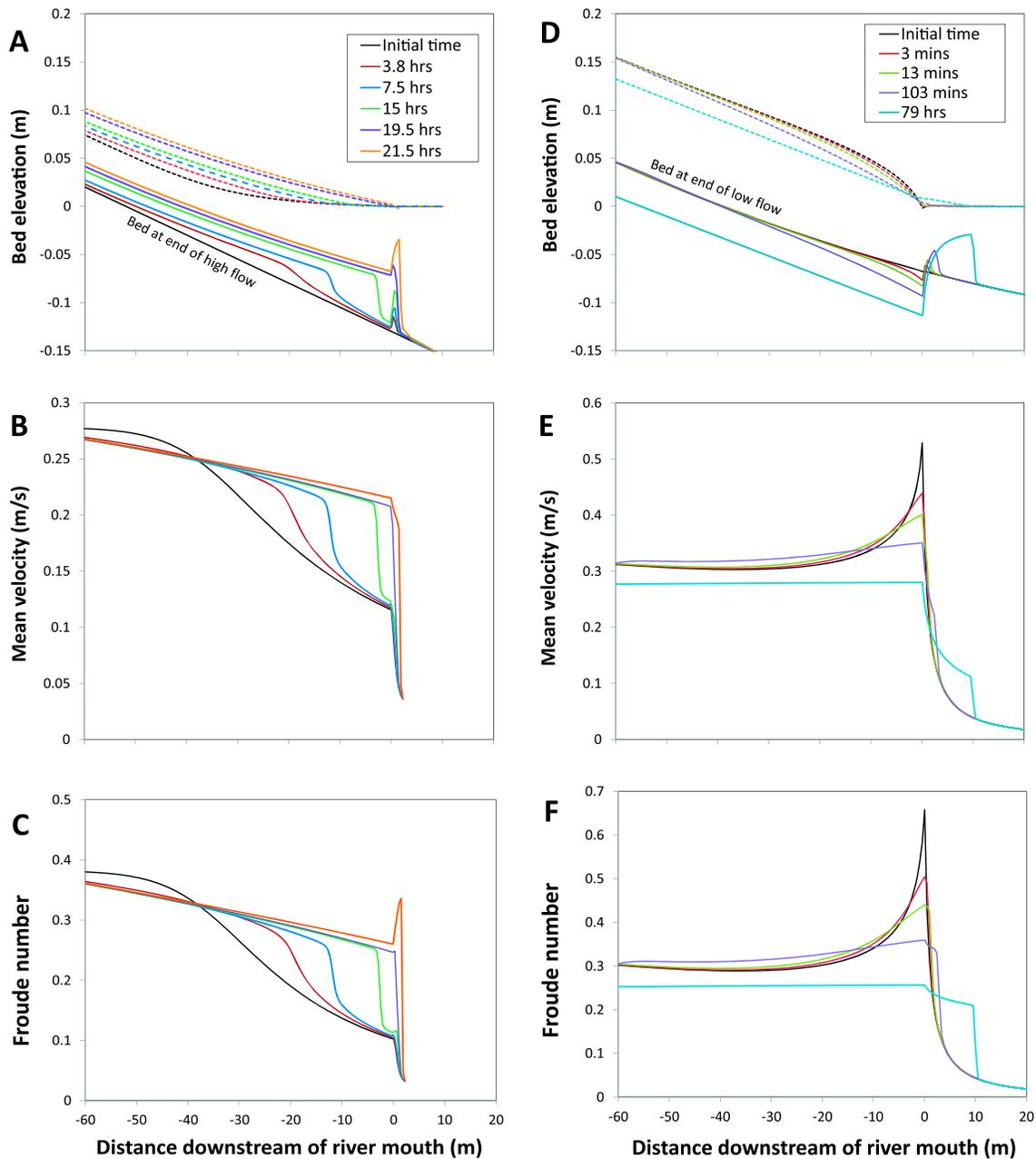
**Figure 4.** Numerical model results for (a–c) low-flow transient run, and (d–f) high-flow transient run. The plots include bed (solid lines) and water surface (dashed lines) elevations as shown in Figures 4a and 4d, mean flow velocity as shown in Figures 4b and 4e, and Froude number as shown in Figures 4c and 4f. Numerical model used the sediment-deposit and plume spreading angles measured in the experiments (Table 1).
