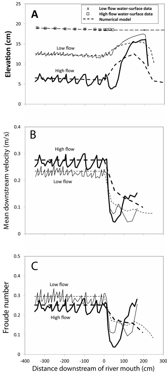
**Figure 5.** Experimental results along the flume centerline from the equilibrium runs for low-flow and high-flow conditions (Experiments 1 and 2) showing (a) bed and water surface elevations, (b) average flow velocity, and (c) Froude number. Dashed lines are from the numerical model and solid lines are the flume results. Flow is from left to right. The vertical axis is referenced to the flume bottom.
