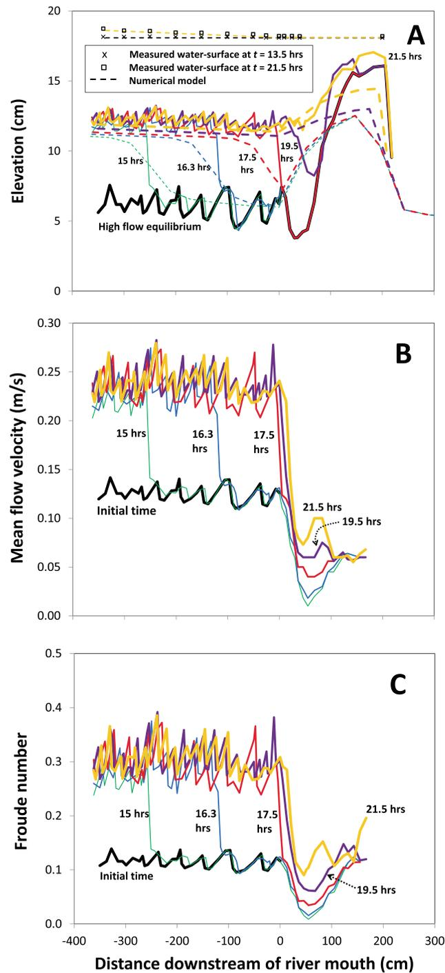
**Figure 7.** Experimental results from Experiment 3 (low-flow transient; solid lines) starting from high-flow equilibrium conditions (black lines) for (a) bed and water surface elevations, (b) mean flow velocity, and (c) Froude number. Dashed lines are from the numerical model. Flow is from left to right. The vertical axis is referenced to the flume bottom.
