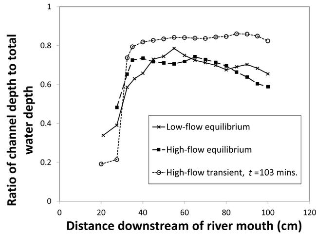
**Figure 10.** Plot of the ratio of channel depth (difference between levee top and thalweg elevation) to total water depth (difference between the water surface and the thalweg depth) along the plume centerline in the offshore basin for Experiments 1, 2, and 4. The values from Experiment 3 are omitted here since they are similar to Experiment 2.
